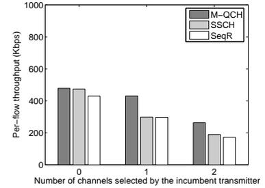
Figure 6: Throughput of non-disjoint flows with incumbent traffic.
