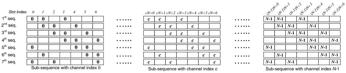
**Figure 2: An L-QCH system,  $Q$ , with  $m = N$  rendezvous channels and  $\tau = 7$ . To construct  $Q$ , we use a minimal cyclic quorum system  $S = \{\{0, 1, 3\}, \{1, 2, 4\}, \{2, 3, 5\}, \{3, 4, 6\}, \{4, 5, 0\}, \{5, 6, 1\}, \{6, 0, 2\}\}$  under  $U = \mathbf{Z}_7$ . The channel indexes for “blank” slots are randomly selected from  $[0, N - 1]$ . Any two sequences in this system overlap on all  $N$  channels.**
